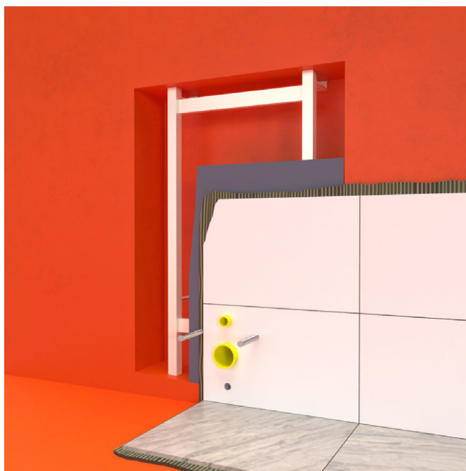
FIGURE 23. Watertight membrane behind built-in WC in wall
