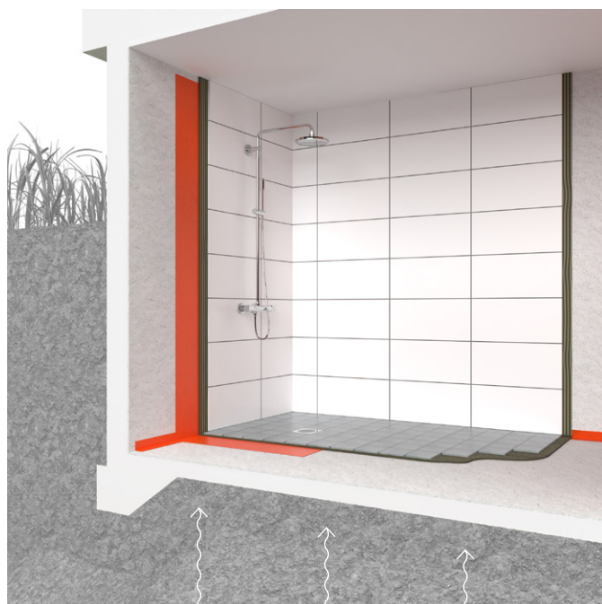
FIGURE 2. Basement with ground moisture penetration
